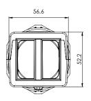
OSF 50 is a divisible cable gland with metric thread especially designed for cables with connectors.
